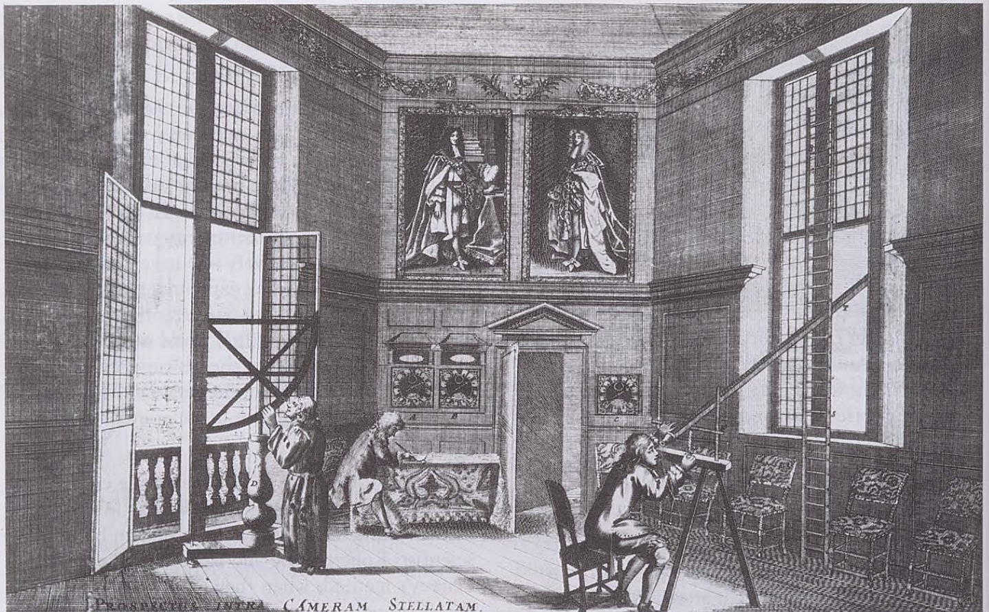
The Royal Observatory at Greenwich was founded by Charles II, who had a great interest in scientific matters. On the left a quadrant is being used, larger but similar to those used for navigation on ocean-going ships. On the right an extremely long telescope is being used to observe the heavenly bodies.
